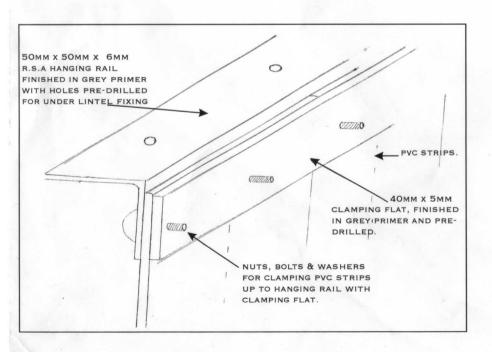
THE STRIPS ARE MANUFACTURED FROM HIGH QUALITY EXTRUDED PVC, HAVING ROUNDED EDGES FOR SAFETY. THE PVC HAS A HIGH TENSILE STRENGTH, IS NON-COMBUSTIBLE AND SELF-EXTIGUISHING. THE STRIPS CAN BE ARRANGED TO SUIT ANY OF THE OVERLAP PATTERNS SHOWN BELOW.
